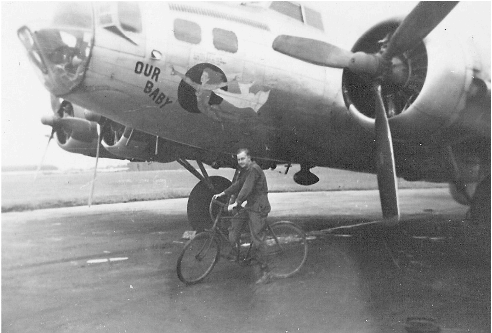
aircraft with chin turret removed for project Casey Jones
