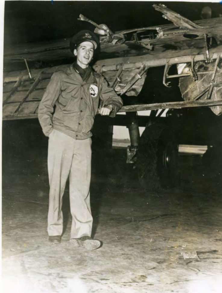
Bomb damage sustained over Hannover 26 Jul 43. Left aileron torn away by bomb dropped by another forma- tion. Lt. Dudley Fay pictured.
